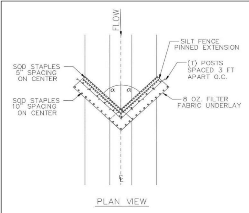
**Figure CD-6 Silt Fence Check Dam Plan View**
