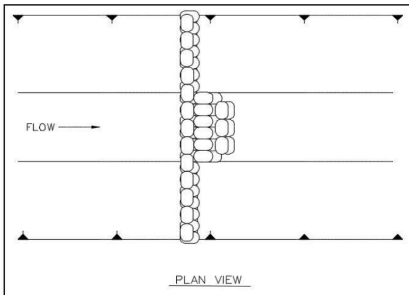
**Figure CD-9 Sand Bag Check Dam Plan View**
