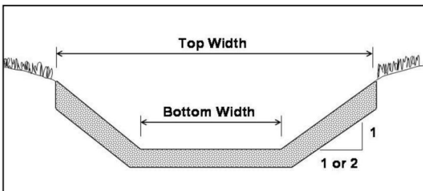
**Figure LS-1 Concrete Lined Swale**
