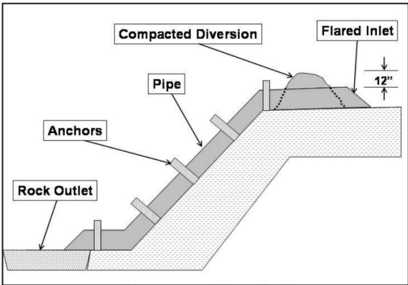
**Figure TSD-1 Temporary Slope Drain**
