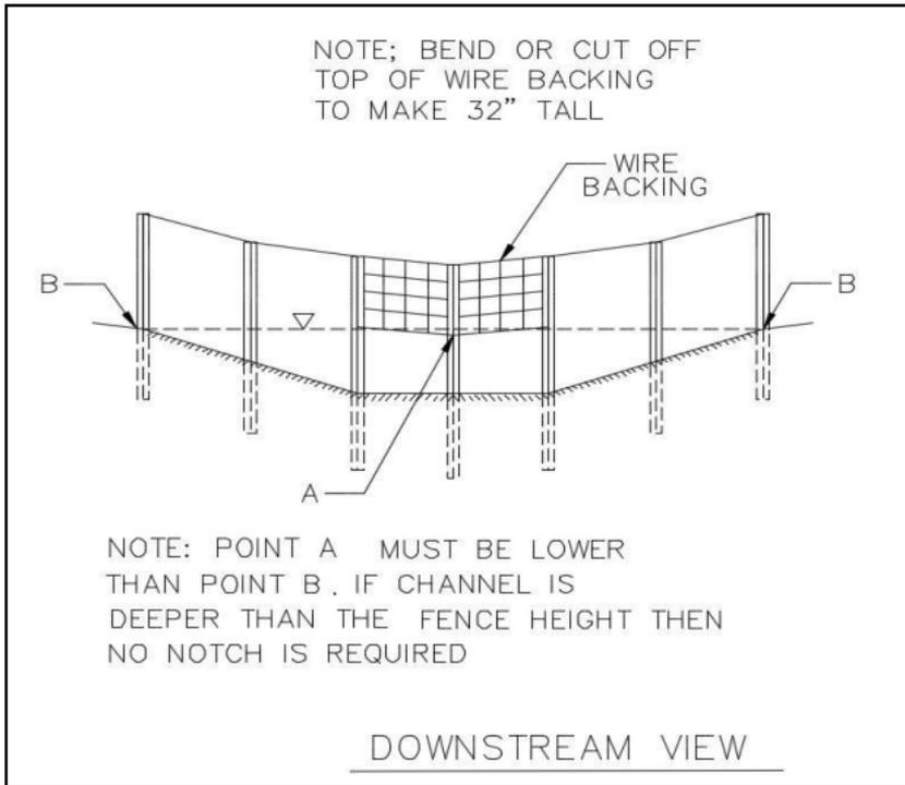
**Figure CD-5 Silt Fence Check Dam Cross-Section**
