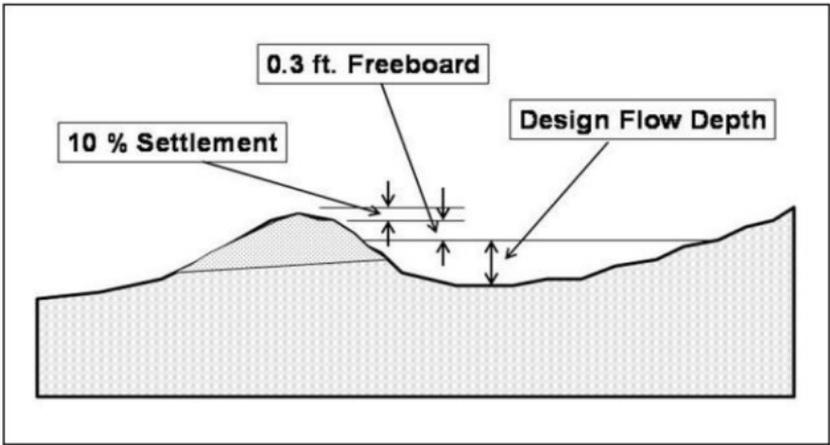
**Figure DV-1 Typical Parabolic Diversion**
