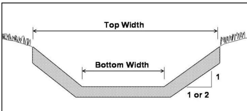
**Figure LS-1 Concrete Lined Swale**
