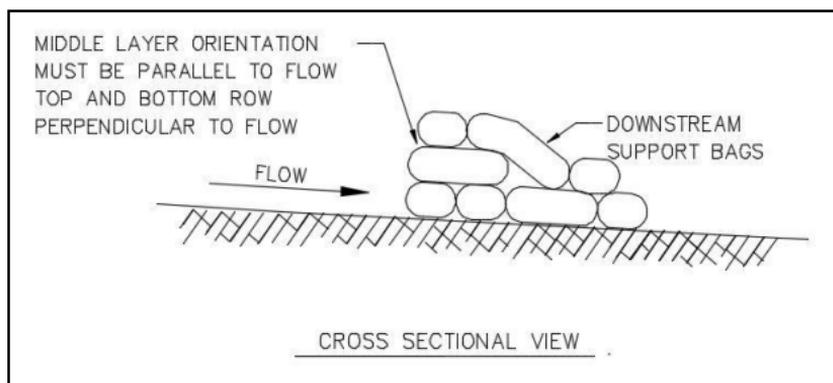
**Figure CD-8 Sand Bag Check Dam Cross-Section**
